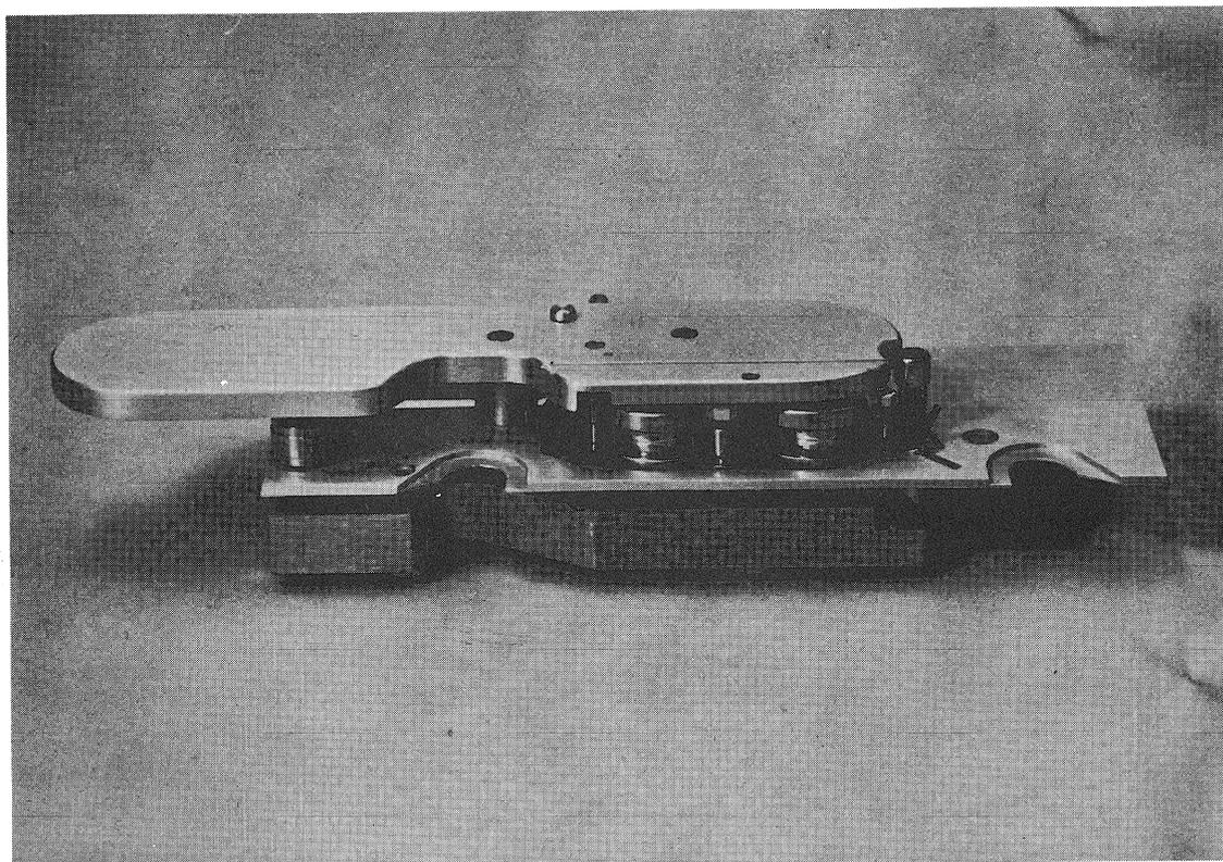
Owing to the shorter distance between the record and the reproduce head the scrape flutter idler had to be redesigned. However, these changes had no negative effects on its performance parameters.
